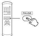
Press the PAUSE button to pause playback (the ring surrounding the PAUSE button on the main unit lights). Press PLAY or PAUSE to restart playback.
